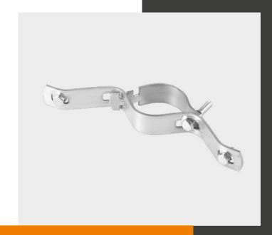
The universal wave holder is an element used for the simple installation of traffic signs. It is made of galvanized steel. This type of holder is designed for signs with reinforcement (bar or rail) on the back of the sign. The holder is first attached to the sign and then to the post.
